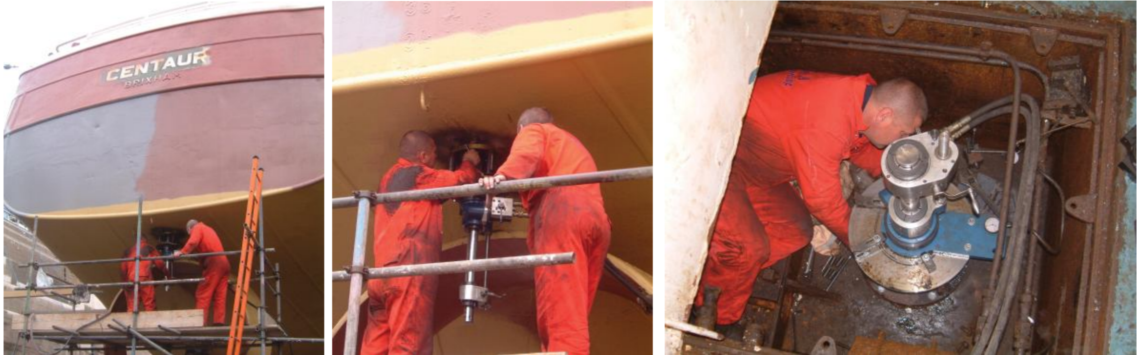
Tight access to this rudder bore is not a problem for M & A engineers when utilising one of our smaller range of line boring equipment.
