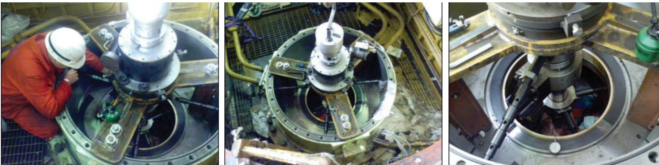
Machining the upper ring of a rudder bore in-line with the lower rudder bore location.
