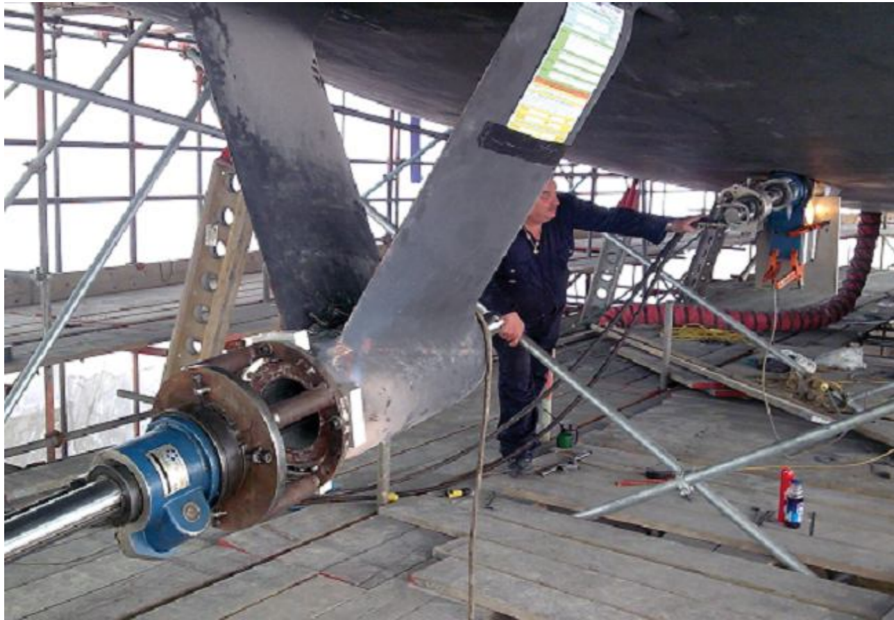
By utilising two sets of equipment, the 'A' frame bore, and Stern Tube bore, could be machined simultaneously.
