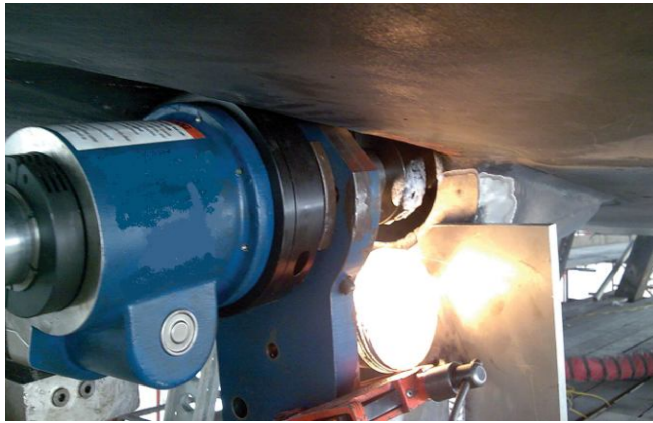
By utilising two sets of equipment, the 'A' frame bore, and Stern Tube bore, could be machined simultaneously.
