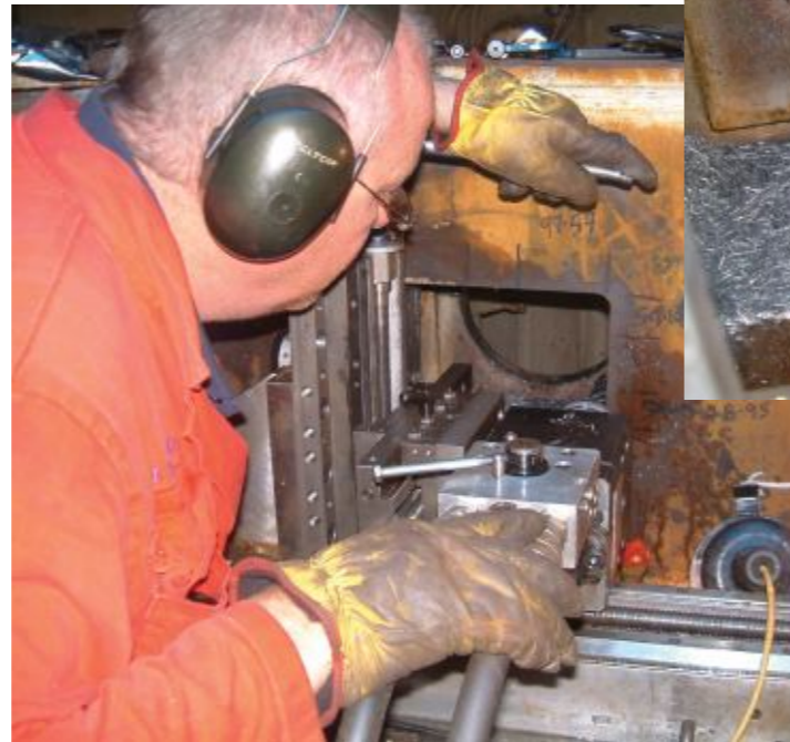
Milling In Progress. Note The Rear Ø240mm Pin Location Bore
