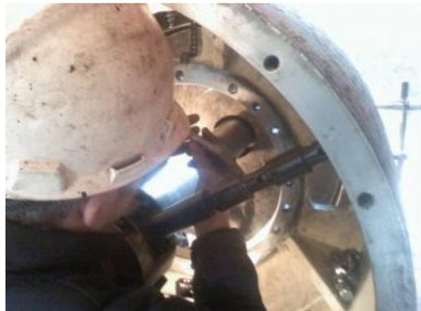
M & A utilised one of its range of heavy duty line boring bars to replicate the position of the Bow Thruster Shaft. When the vertical bar had been set in the drive shaft housing bores, a sweep reading was taken across the horizontal bar. No error was found.
