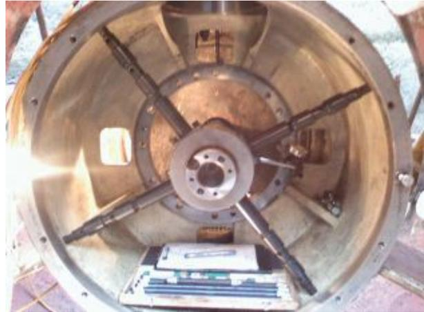
The ships engineers also wished to check the angularity between the Drive Shaft and Bow Thruster Shaft, where the pinion gears mesh.
