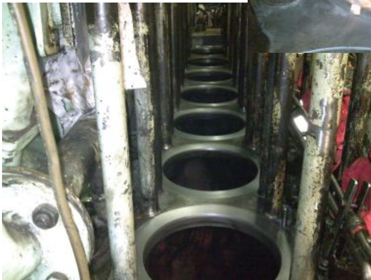
Completed Water Jacket Landings
