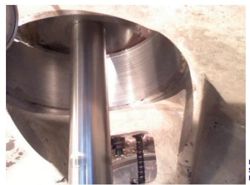
**Machining The** Sleeve To The **Final Size**
